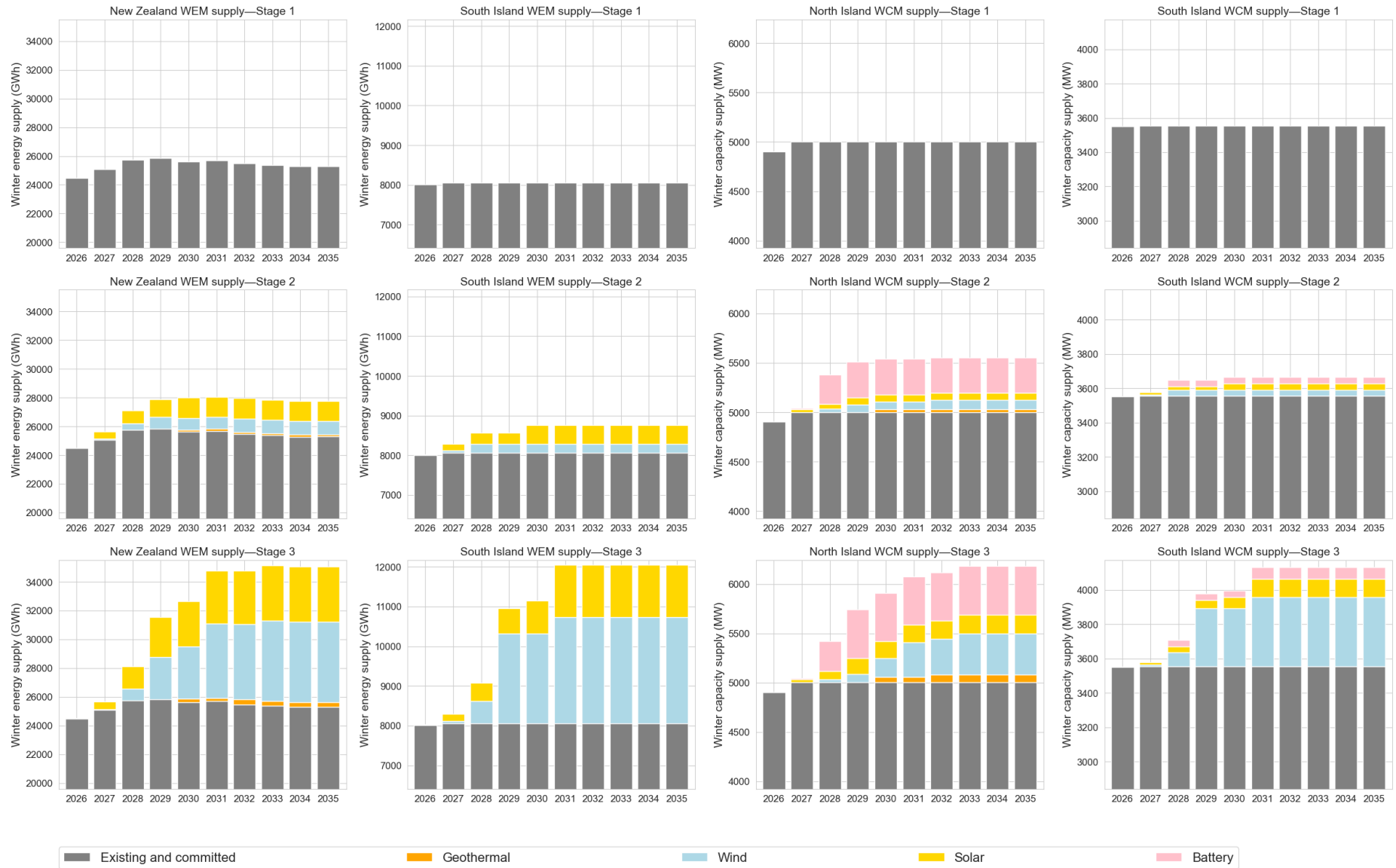
Figure 3: Contributions of supply pipeline to the New Zealand Winter Energy, South Island Winter Energy and North Island Winter Capacity margins
